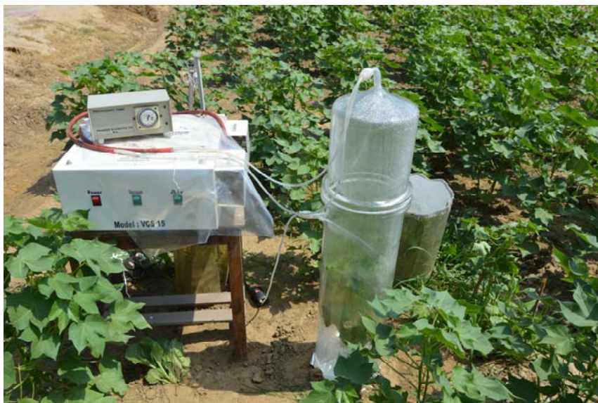
Plate 3.10: Volatile collection from cotton plant through Vacuum Plant Volatile Collection System (Mascot Enterprises, VCS-15)
